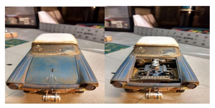
Thanks to Tom Geiger at Model Car forums, who noted in the WIP Drag car threads to make sure the rust does not look like it was streaked on with a brush. I used circular motions with sandpaper to remove the streaks. The 2 tone interior color is the Aeromaster Russian light blue with very nice kit fabric decals on the old skool bench seat (GM P.E. seatbelts added) and interior doors. Then the dust was applied to the interior and the floor got plenty of rust.
