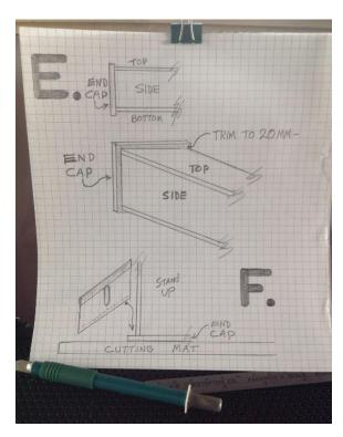
After gluing the top and bottom to the sides (the sides are the smaller pieces) we now glue the oversize end pieces to our box as in illustration E. We do not have to be 100% precise on the ends because they are larger than needed. When the glue has dried (with liquid cement it should only take a few minutes) we can use a craft knife or a razor blade to remove the excess from the end caps as shown in illustration F. This construction method is the basis for most scratch building.
