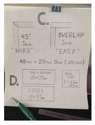
In illustration D you can see the dimensions of our  $40 \times 20$  box are both smaller and larger than our finished product. That is because we must take into account the thickness of the plastic sheet we are using. With the overlap joint we must reduce the size of the side pieces because the top and bottom will overlap, we must also reduce the overall length of all pieces because of the end caps ,which are cut larger to make it easier to assemble.
