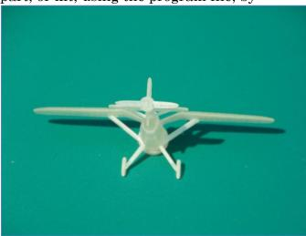
"spinning" it out in an additive process with melted threads of media, such as nylon. It's the spinning feature that affords the technology the ability to provide a hollow detailed interior in the finished product.
