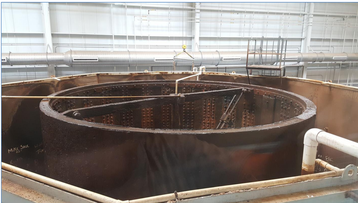
The turret shell in the drained preservation tank. The turret is 20' in diameter, 9' high.
