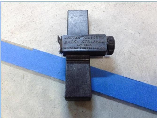
Normally this tool is used by balsa flying model builders but I've found that it works great on thin sheet plastic up to .030". You just set the width of your cut by turning a knob on the side of the tool. You place your cutting material on a straight edge and then
